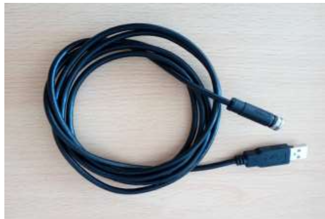
Figure 2: USB to M8 cable
