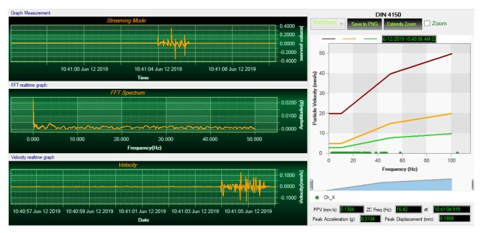
Figure 46: Velocity and FFT Graph, PPV and PVS
