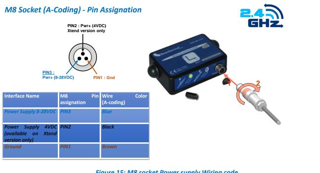
Figure 15: M8 socket Power supply Wiring code
