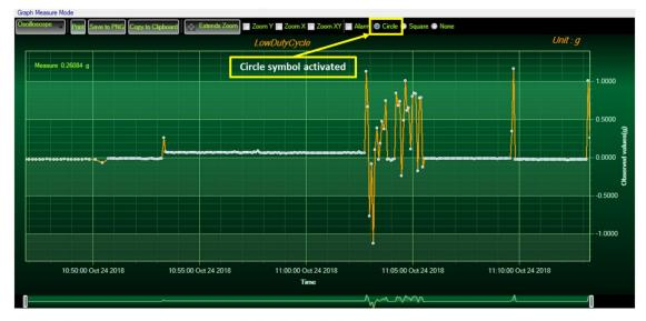
Figure 74: Graph measure mode: Frame Marks
