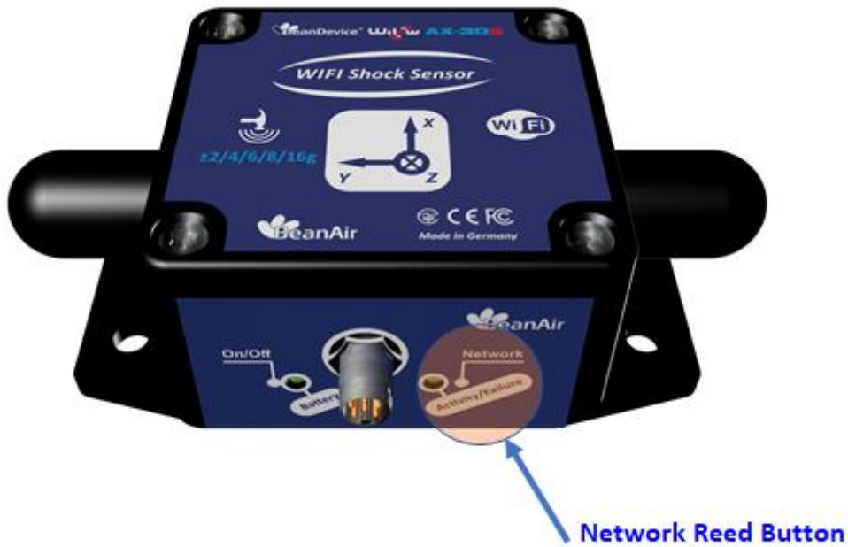
Figure 192: Network Reed button position
