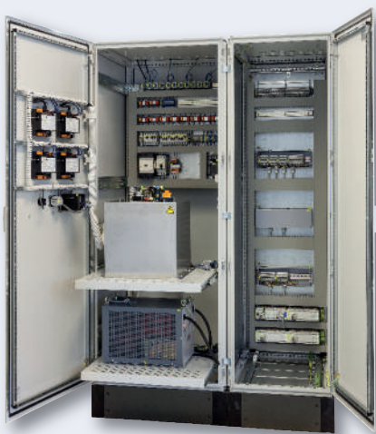
Complete testing system for testing of household appliance
