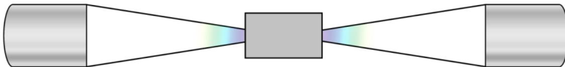
This is used when 2 confocal probes are used in opposition to each other for measuring changes in thickness.
