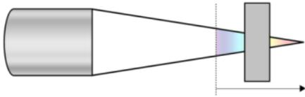
This is used for either measuring both sides of a transparent object or the thickness (note: if the transparent object is thicker than the range of the probe, then the Single head distance measurement instructions should be used).
