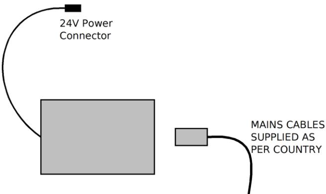
1. Connect the 24 V power supply connector to the confocal unit and plug power block into the mains cable provided.
