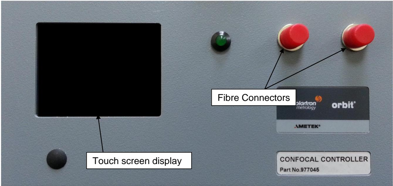
1. Remove the dust cap from the Fibre Connector on the controller (pull off).
