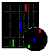
Cluster pixel defect type 3a Sub-pixels in a cluster area constantly lit
