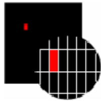
Pixel defect type 3a Sub-pixel/dot (red, blue, green) constantly lit
