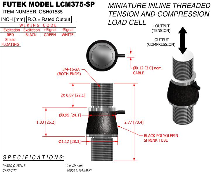
SAFE OVERLOAD 150% of R.O. ZERO BALANCE ±3% of R.O. EXCITATION (VDC OR VAC) 18 MAX BRIDGE RESISTANCE  $350 \Omega$  nom **NONLINEARITY** ±0.5% of R.O. HYSTFRESIS ±0.5% of R.O. *NONREPEATABILITY* ±0.1% of R.O.
