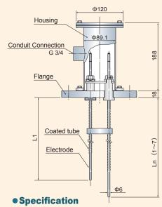
Diameter of Electrode:  $\Phi6/8/10/15/20$ mm
