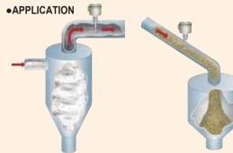
Detect the clog of cyclon Detect failure of baghouse
