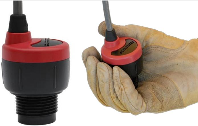
The general purpose ultrasonic level switch provides continuous level detection up to 49.2" (1.25m) with 4 programmable relays for level switch or level control functions, and is configured via our free WebCal software. The embedded level controller can lower cost by replacing external control hardware. This non-contact liquid level sensor is ideally suited for corrosive, sticky or dirty liquids, and is broadly selected for small day tank, skid, IBC, sump and process tank level applications.
