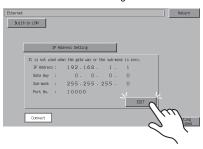
Change the IP address using the keypad.
