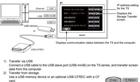
Load screen data from the computer into storage in advance. Press the [Storage (English)] switch on the initial screen. The Storage (English IP Address (English)
