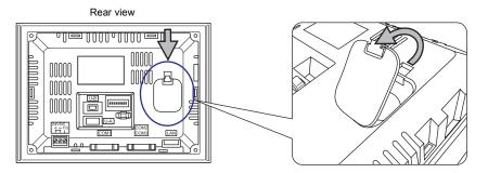
4. Press the detent on the right of the battery in the direction of the arrow.
