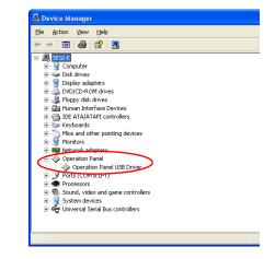
This will disappear when MONITOUCH and computer are disconnected. If [Other Device] or a mark other than shown above is displayed even while the USB is connected, the USB driver is not recognized. If this happens, uninstall the USB driver and reinstall it.
