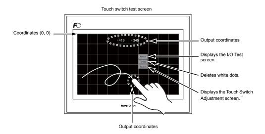
\* If a position different from the pressed position turns white, refer to "Touch Switch Adjustment" on the next page and adjust the touch switch position.
