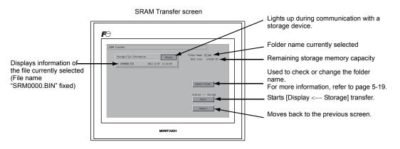
Transfer or comparison start Check [Folder Name], [Rest Size], and the transfer direction. Press the [Start] switch. During data transfer or comparison, the [Start] switch changes to [Transferring].
