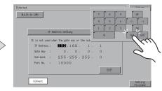
It is not used when the gateway or the subnet mask is zero.
