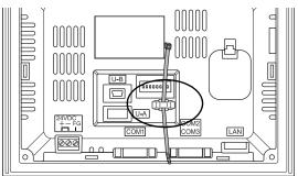
Inserting and securing a USB cable Insert a USB cable and secure it using the cable tie.
