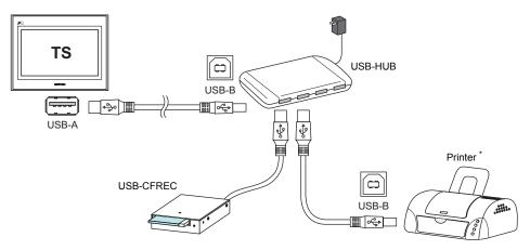
\* A parallel printer can also be connected (on conditions that the model is available with the TS series and connected with a commercially available parallel-to-USB cable (ELECOM's UC-PGT recommended)). For more information on available printer models, visit our website (http://www.monitouch.com).
