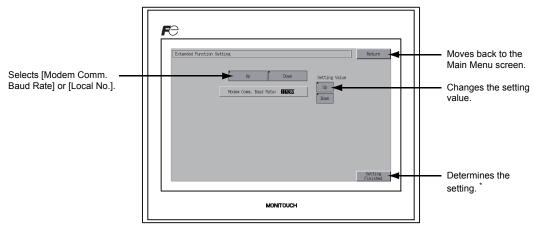
\* The switches on the Main Menu screen are not valid for 15 seconds after the [Setting Finished] switch is pressed.
