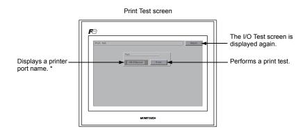
\* The printer port name specified on the V-SFT-5 editor is displayed. Either [USB-A (Host)] or [USB-B (Device)] is displayed.
