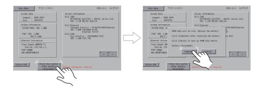
9. Check that the [Press this switch after battery replacement.] switch and the message "Battery changeover required" are cleared from the bottom of the Main Menu screen.
