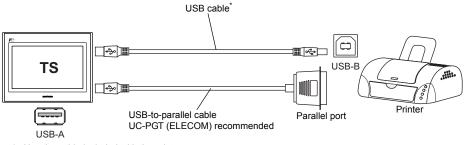
\* Use the cable included with the printer.
