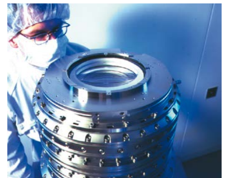
Capacitive displacement sensors measure with the highest precision the alignment of the lens system used for semiconductor wafer lithography.
