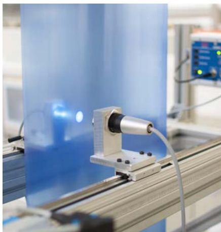
Inline colour gradient measurement of transparent film and acrylic glasses.
