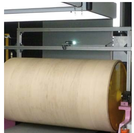
Colour measurement of continuous strip coating such as aluminium, zinc and paper during production.
