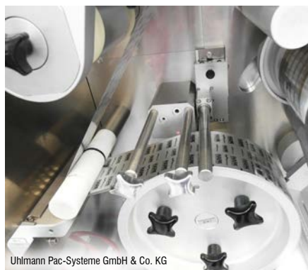
Foreign body detection in medical technology MDS sensor recognises foreign bodies in blister machines during the tablet packaging process.
