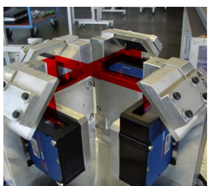
Measuring system detects the XY position of the needle in an industrial sewing machine
