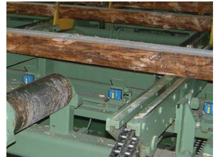
optoNCDT on trimming systems of saw mills
