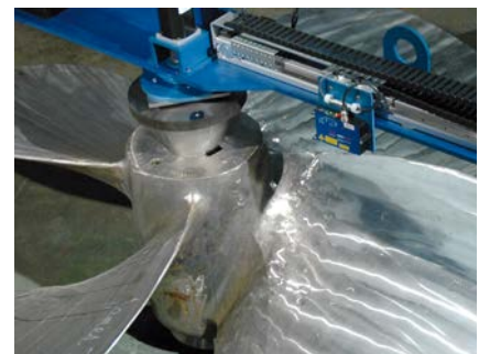
Profile measurement of marine propellers
