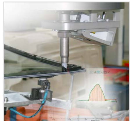
Inspection of the adhesive beading
