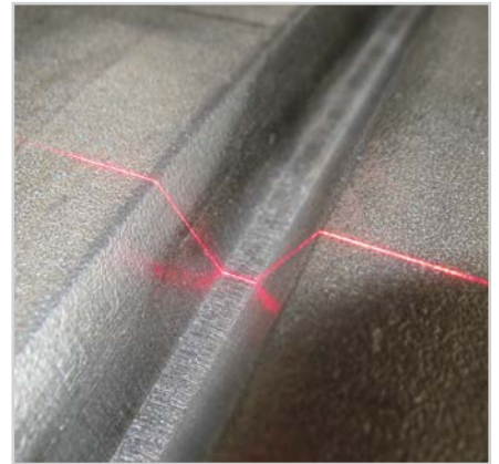
V-gap measurement on pipes
