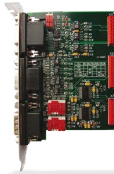
Interface card IF2008, IF2008E for individual signal processing
