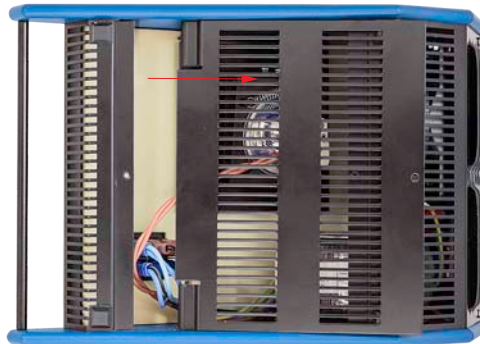
Fig. 8 Remove the bottom cover
