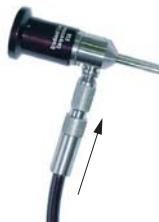
Fig. 8 Connecting the fiber optic cable to an endoscope
