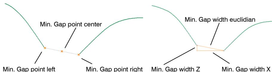
Fig. 4.34: "Advanced Basic Gap" measured values, "Min. Gap"
