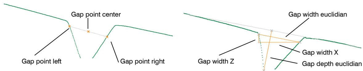
Fig. 4.21: "Flat Groove Gap" measured values, "Gap" group
