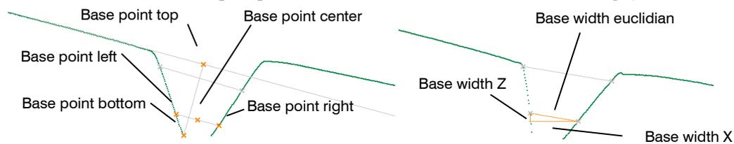
Fig. 4.48: "Advanced Groove Gap" measured values, "Base" group
