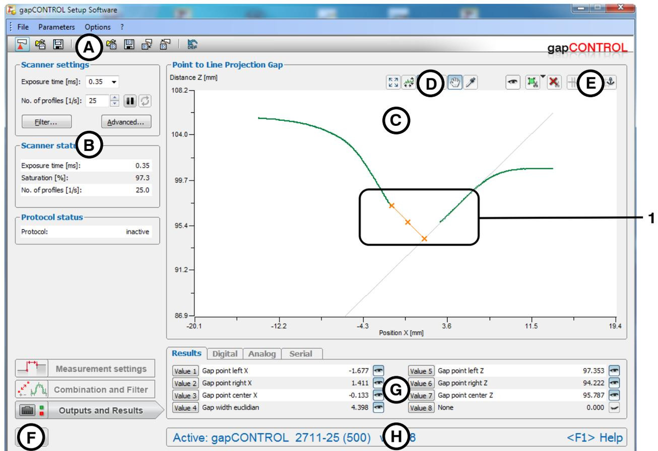
Fig. 4.15: "Point to Line Projection Gap" measuring program ("Point to Line left" algorithm)
