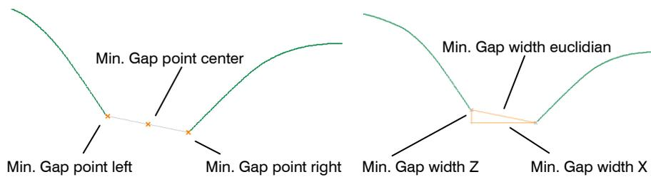
Fig. 4.40: "Advanced Projected Gap" measured values, "Min. Gap"
