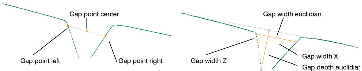
Fig. 4.45: "Advanced Groove Gap" measured values, "Gap" group
