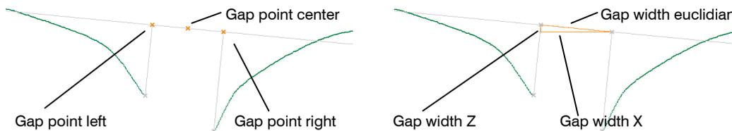
Fig. 4.14: "Double Line Projection Gap" measured values
