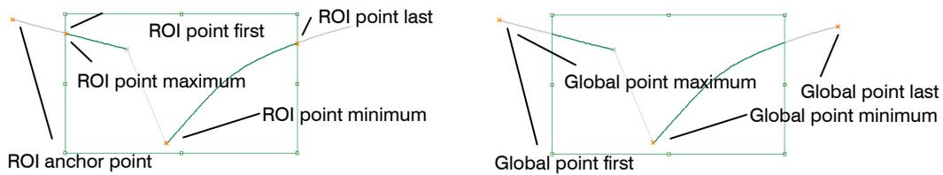
Fig. 4.35: "Advanced Basic Gap" measured values, "ROI" and "Global" groups
