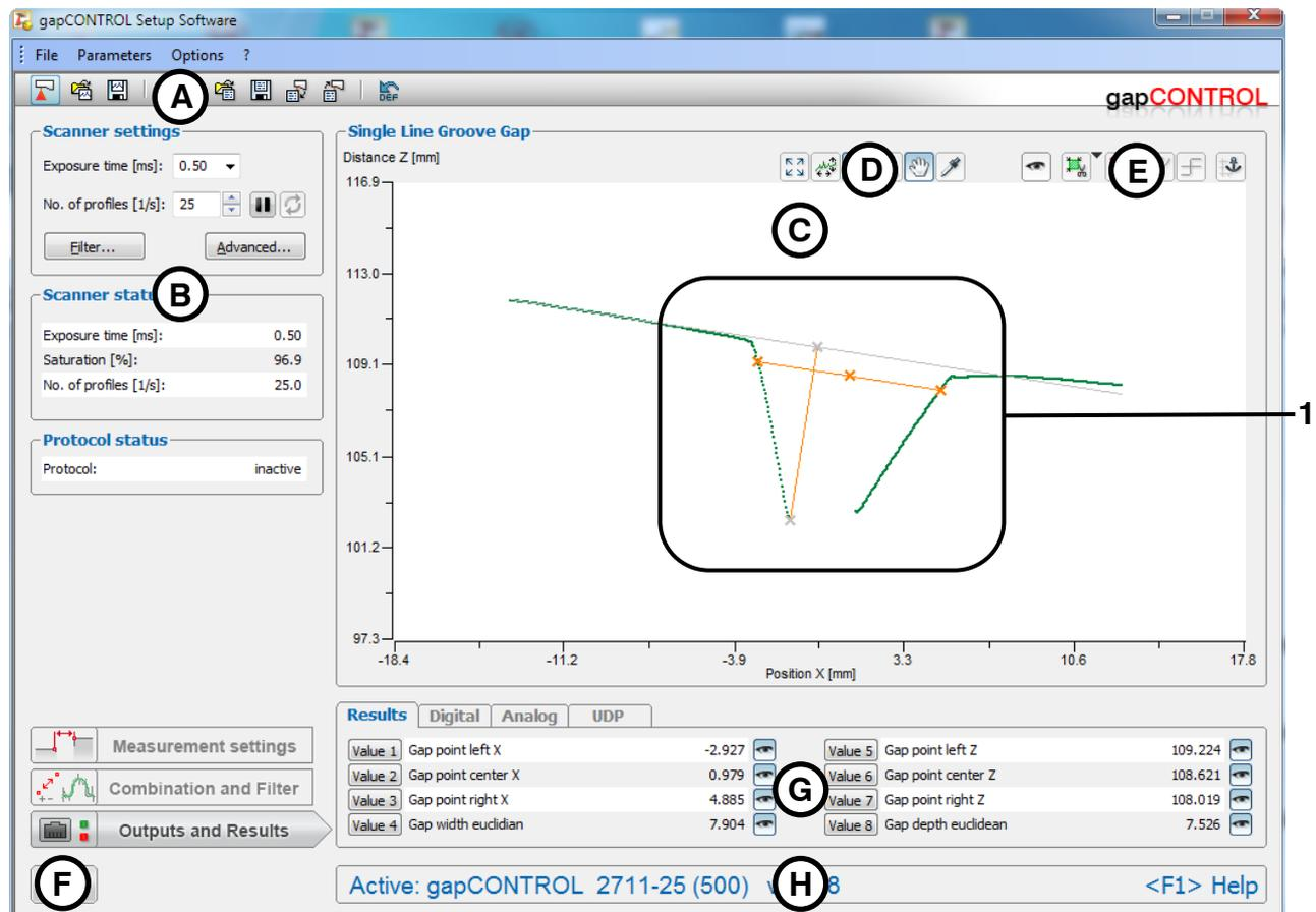
Fig. 4.27: "Single Line Groove Gap" measuring program
