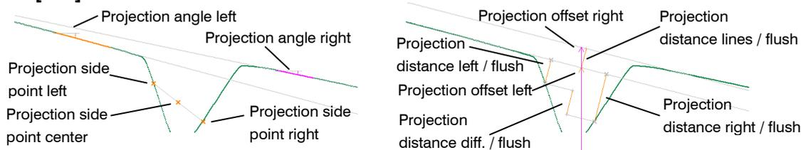
Fig. 4.47: "Advanced Groove Gap" measured values, "Projection" group
