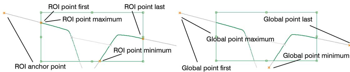
Fig. 4.49: "Advanced Groove Gap" measured values, "ROI" and "Global" groups
