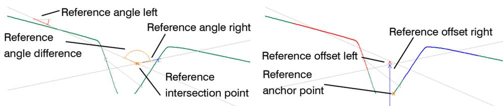
Fig. 4.46: "Advanced Groove Gap" measured values, "Reference" group
