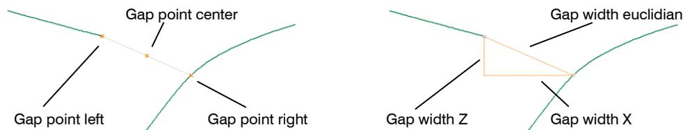
Fig. 4.31: "Advanced Basic Gap" measured values, "Gap" group
