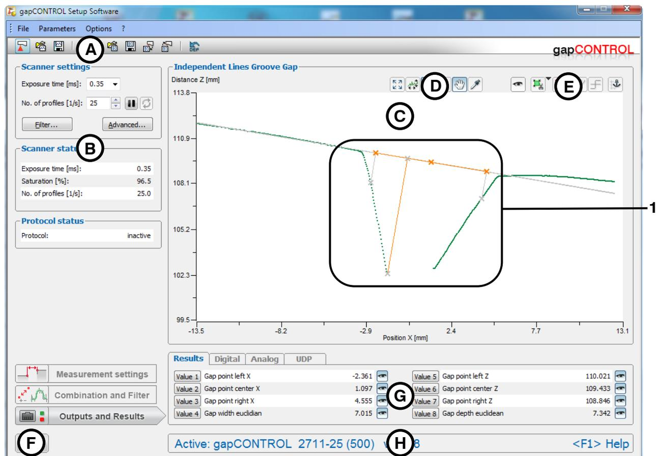
Fig. 4.25: "Independent Lines Groove Gap" measuring program
