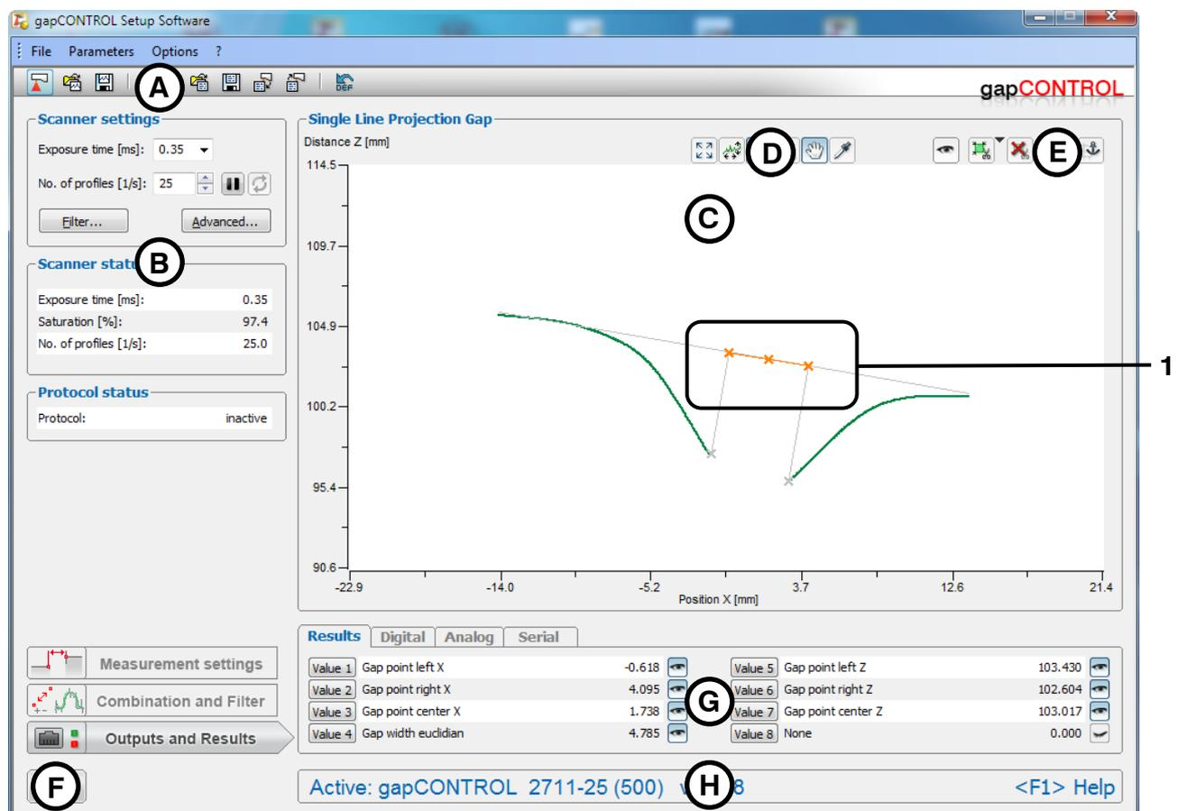
Fig. 4.11: "Single Line Projection Gap" measuring program
