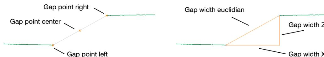
Fig. 4.3: "Edge Points Gap" measured values
