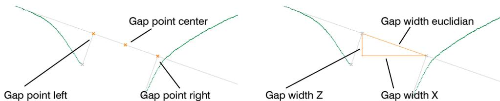
Fig. 4.12: "Single Line Projection Gap" measured values
