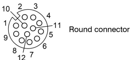
Fig. 7.1: gapCONTROL 2611/2911 trigger input (RS422 interface half-duplex and digital input, view on solder pin side of connector)
