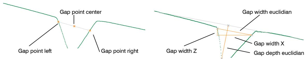
Fig. 4.26: "Independent Lines Groove Gap" measured values, "Gap" group
