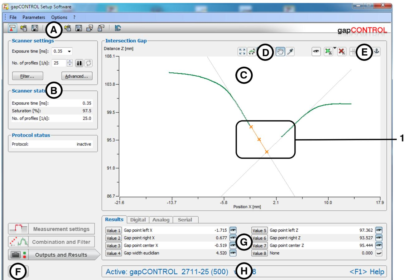
Fig. 4.17: "Intersection Gap" measuring program ("Intersection left" algorithm)
