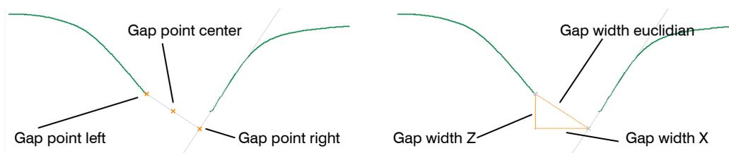
Fig. 4.16: "Point to Line Projection Gap" measured values
