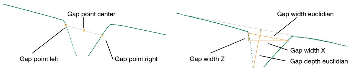
Fig. 4.28: "Single Lines Groove Gap" measured values, "Gap" group
