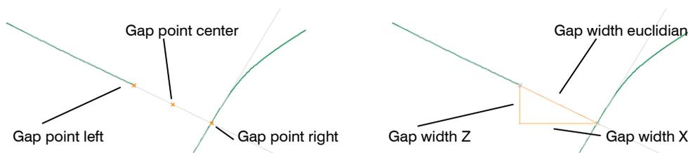
Fig. 4.37: "Advanced Projected Gap" measured values, "Gap" group
