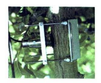
Our OEM makes an adapted fixture to fix the LVDT directly on the samples. The tests could be also engaged directly on the field, everywhere on the globe. The communication will be handled by a low power consumption electronics, including a GPRS transfer mode.
