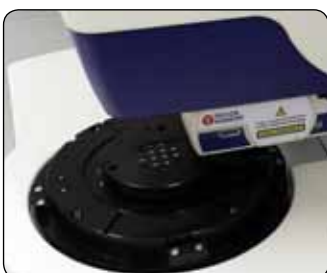
Batch testing of multiple parts
