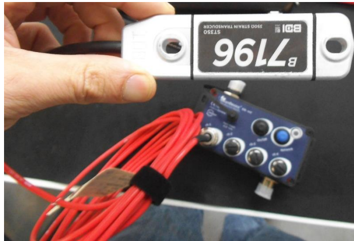
Load strain transducer combines with the Beandevic AN-mV
