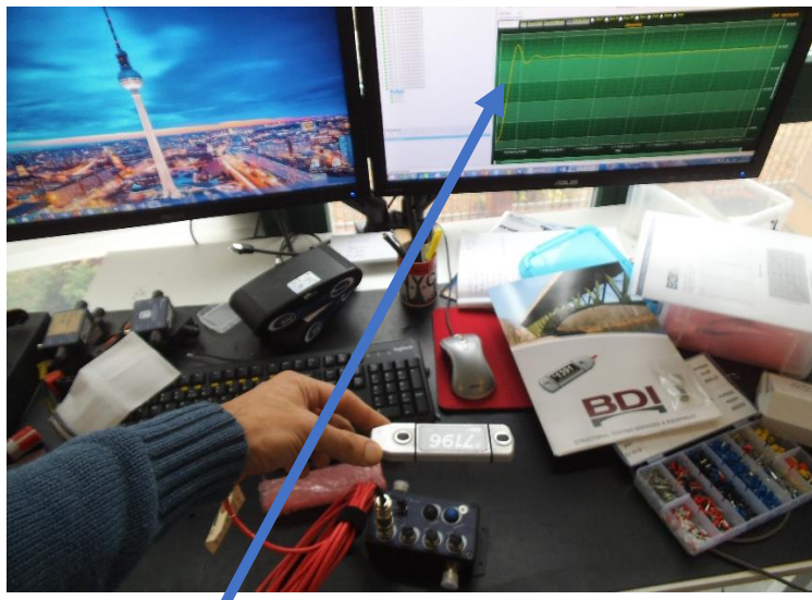
Load strain transducer combines with the Beandevic AN-mV
