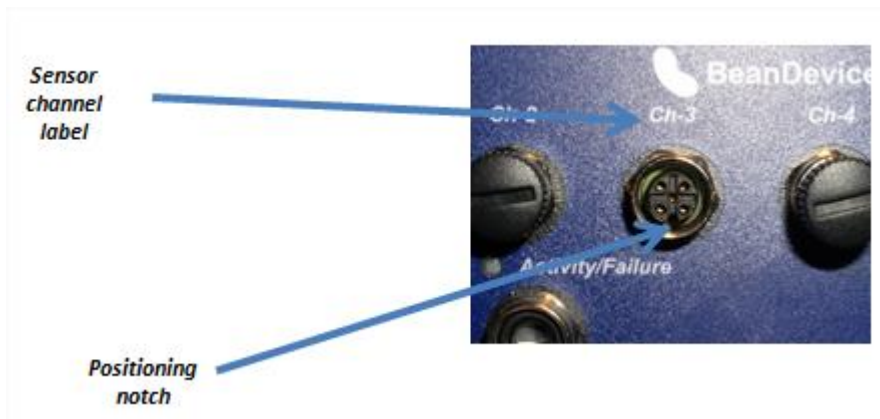
Figure 6: M12 Socket - positioning notch
