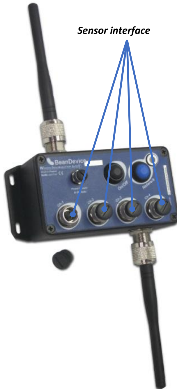
Figure 5: M12 socket location the BeanDevice®
