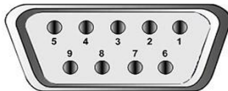
Figure 7: Serial line wiring code (RS232/RS485)
