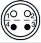
Fig. 3 Pin assignment connector USB port
