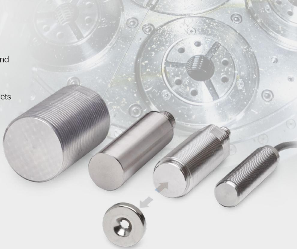
mainSENSOR distance sensors use an innovative measuring principle, which combines the advantages of both inductive and magnetic sensors. Measuring the distance to a magnet which is attached to the measuring object, the sensor outputs a continuous, linear output signal. By using magnets of different strengths, measuring ranges between 20 mm and 55 mm can be achieved. In order to adapt the measuring range, you only have to change the magnet.
