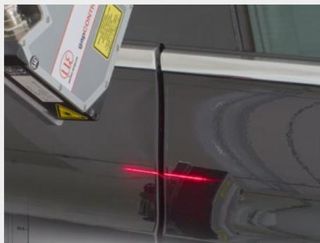
Gap and flushness measurement on bodywork parts
