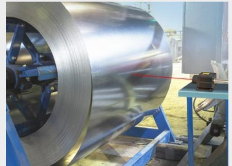
Acquisition of coil diameters
