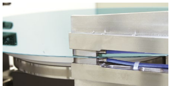
Wafer thickness measurement with two capacitive sensors
