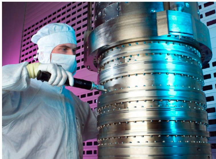
Capacitive displacement sensors are used for adjustment with nanometer precision of lenses in optical systems for wafer exposure.
