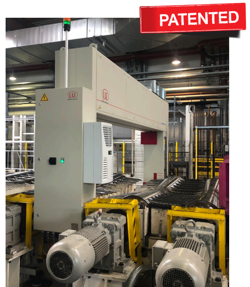
Patented frame-in-frame technology with integrated reference frame to compensate for temperature-induced effects
