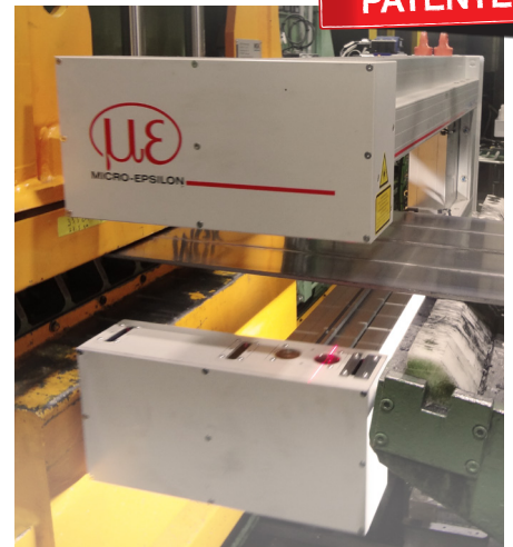
Additional measurement of width and cambering with patented compensation of tolerance-induced effects
