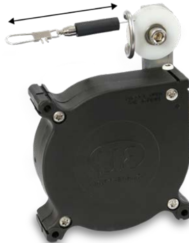
MK88 Sensor mechanics to monitor telescopic booms ▪ Integrated deflection pulley made from plastic with secured "wire guidance" ▪ High spring force ▪ IP67 / -40 °C ... 80 °C ▪ Robust plastic housing
