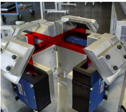
Measuring system for detection of XY position in the sewing machine needle
