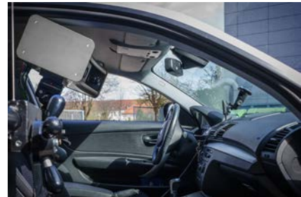
surfaceCONTROL mobile 3D sensor Inspection of the control panel in the vehicle
