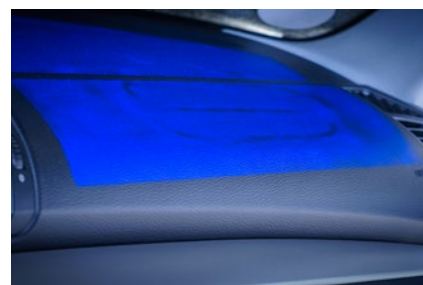
Full-surface back projection of the inspection result
