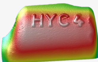
3D text recognition of embossments which cannot be solved with 2D image processing due to lack of contrast
