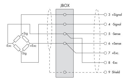
In case of use of two or more load cells, use appropriate junction boxes (CEM4/C or CSG4/C) of which the connection is shown below.
