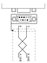
To connect to the Profibus MASTER, use a standard Profibus cable. The typical impedance of the cable should be between 100 and 130 Ohm (f > 100 kHz). The cable capacity (measured between conductor and conductor) should be less than 60 pF/meter and the minimum conductor cross-section should not be less than 0.22 mm<sup>2</sup>.
