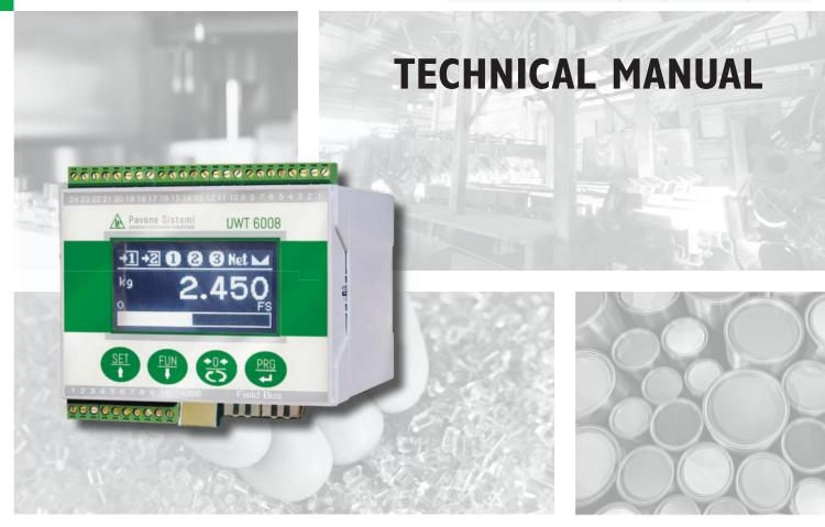
UWT 6008 Weight transmitter/indicator with RS232 serial, analog and Fieldbus output
