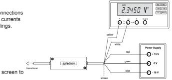
It is usual to connect cable screen to power supply 0 V.
