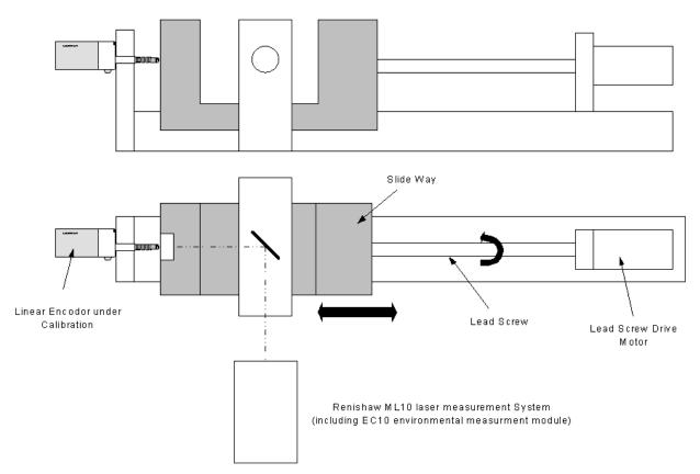
Linear Encoder Laser Interferometer Calibration System
