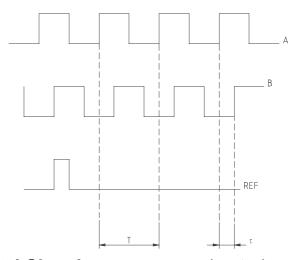
Incremental Signal: are square pulse trains APOS and BPOS, which are phase shifted 90° apart. The inverted equivalent of APOS and BPOS (ANEG and BNEG) are provided for differential applications.
