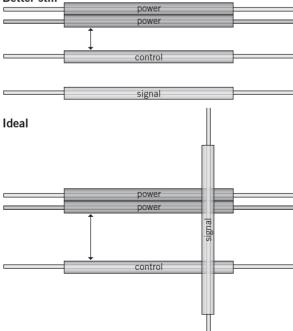
Avoid running cables together e.g. in trunking. When cables are placed closely together even screening can be ineffective. Effects depend on the type and level of interference.
