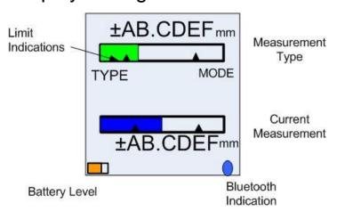
The display can be set to display the range and tolerance of the part being measured. (e.g. 28 ±0.05 mm)
