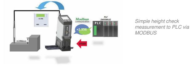
Chip height check with Orbit LT. Measurement sent to PLC on print command via RS232
