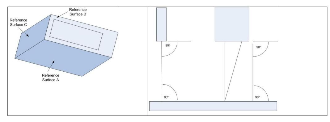
When mounting the head the goal is to have the Reference Surface B parallel as possible to the plane of the target. Take care when using mechanical blocks etc to set up the laser as the window may be scratched.
