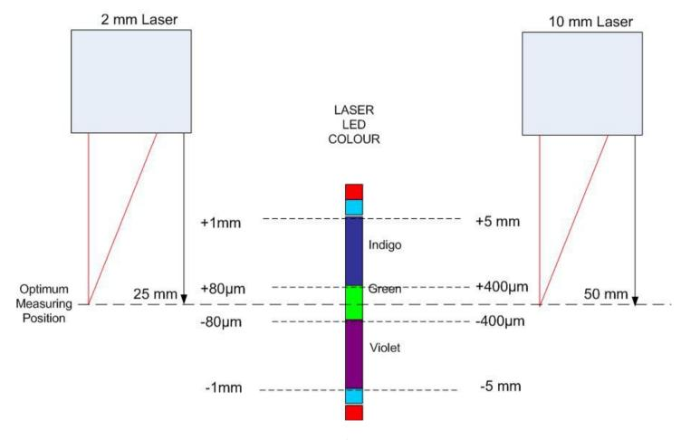
The green led indicates the most accurate position for measurement.
