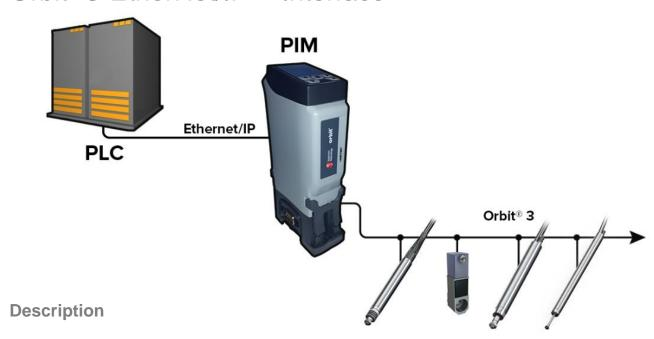
The PIM, is a PLC compatible EtherNet/IP™ to ORBIT®3 interface module, that enable easy connections between any EtherNet/IP™ enabled controller and Solartron's flexible ORBIT®3 digital measurement system.
