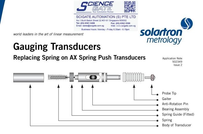
It is advisable when changing springs to make sure that the surrounding area is clean. The smallest particles of dirt trapped in the internal workings of the transducer will have an effect on the stroke.
