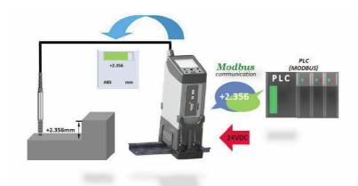
Simple height check measurement to PLC via MODBUS
