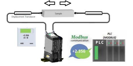
Use 2 S-Series Transducers to monitor a sample under strain
