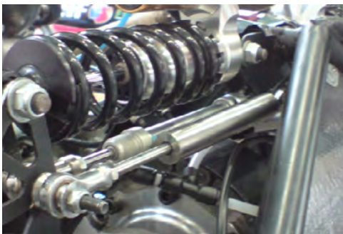
APPLICATION: S-SERIES TRANSDUCER MONITORING AUTO FRAME
