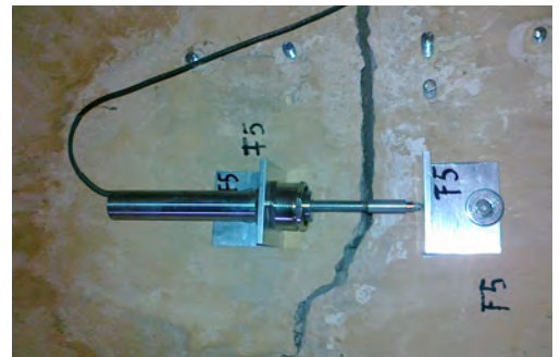
APPLICATION: DISPLACEMENT TRANSDUCER MONITORING A CRACK IN INFRASTRUCTURE
