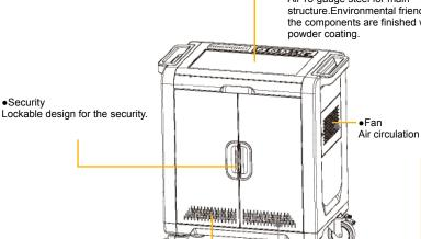
Appearance Unique and durable plastic design. All 18-gauge steel for main Extra Outlet 3 outlets for convenience. Power all structure. Environmental friendly, your peripheries from one standard the components are finished with wall outlet
