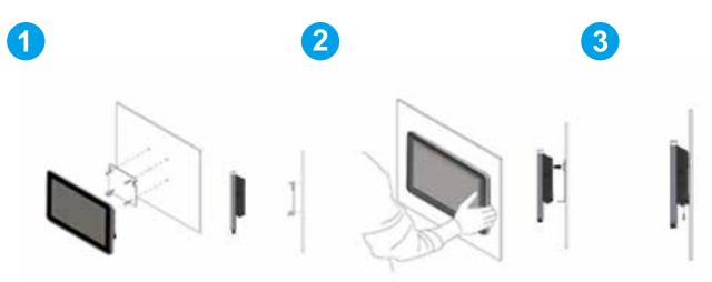
Screw VESA bracket to the fixture (ex. wall) with four M4 x 5 mm flathead screws.
