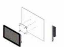
Screw VESA bracket to the fixture (ex. wall) with four M4 x 8 mm flathead screws.
