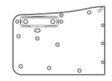
1. Remove expansion port cover from the rear side of M101 Tablet PC.
